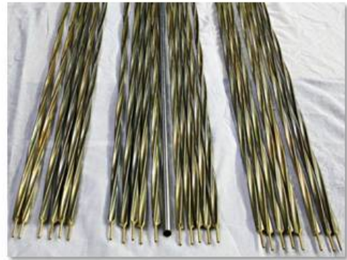
Lightbridge nuclear fuel rods
